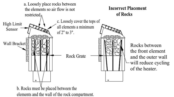
1. Put smaller rocks in first around the outer perimeter of the heating chamber.
