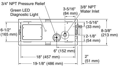
Minimum required access panel is 24" (610 mm) L x 15" (381 mm) H.
