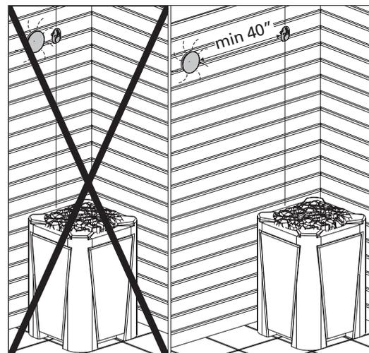
**Figure 10. Sensor's minimum distance from an air vent**
