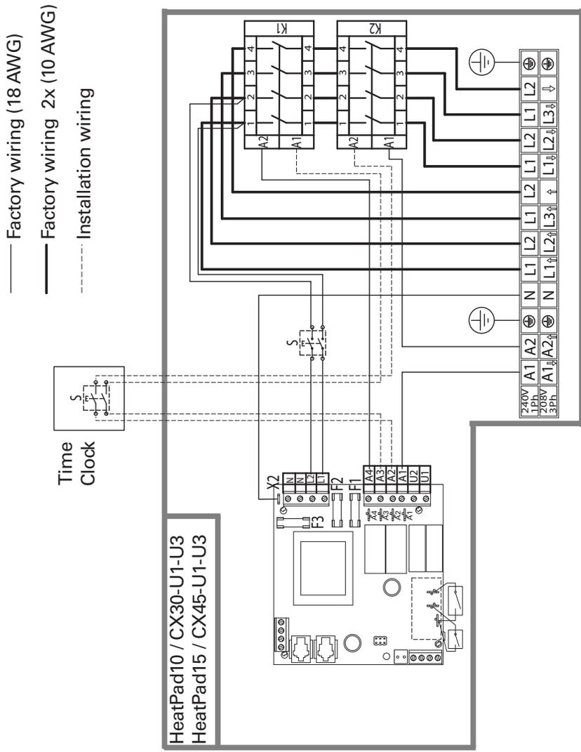
Figure 6.3 Optional Time Clock Electrical Connections (HeatPad10/CX30-U1-U3 and HeatPad15/CX45-U1-U3) for all ProHeat and ClubHeat sauna heater models.
