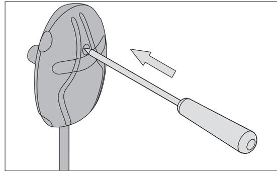
**Figure 11. Reset button of the overheating protector**
