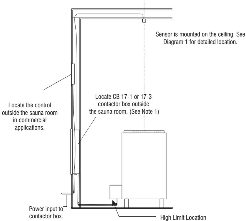
All wiring for sauna system or accessories should be routed inside the walls or away from the high temperature air from the sauna heater.
