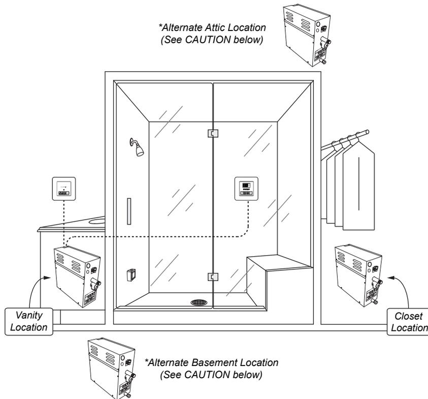
**\*CAUTION:** Steam generators must NOT be installed outdoors, in moist, humid areas, in areas prone to freezing, or extreme heat such as an unventilated attic. To do so will void the warranty.
