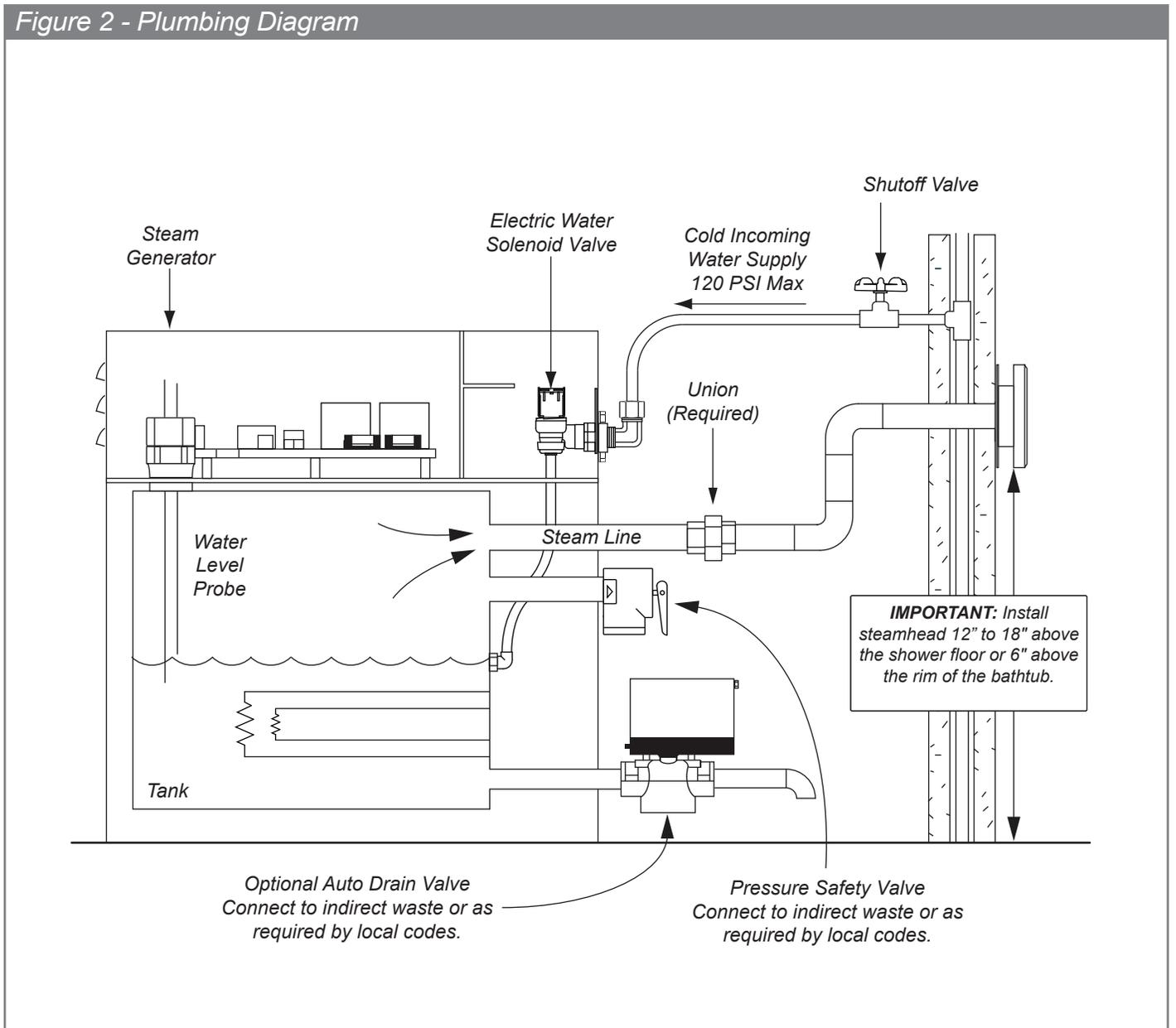
Figure 4 - Typical Installation
