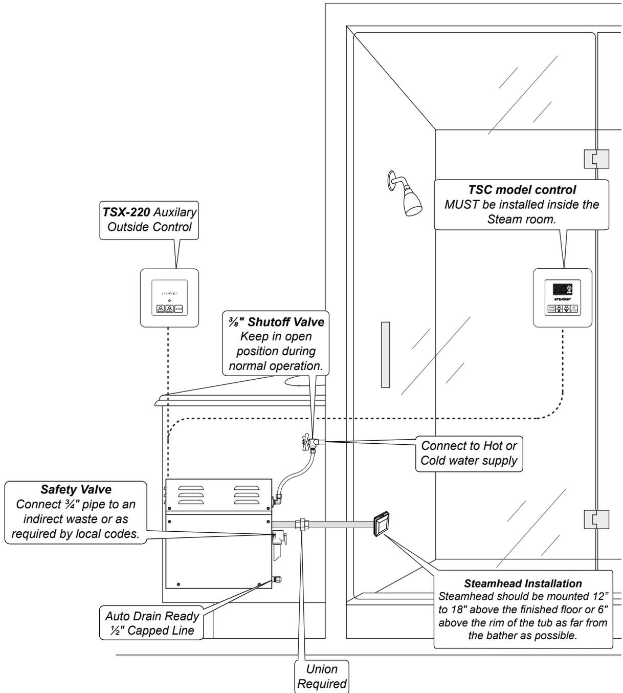
**Steam Outlet Pipe** - Use a 3/4" Copper or Brass pipe.
