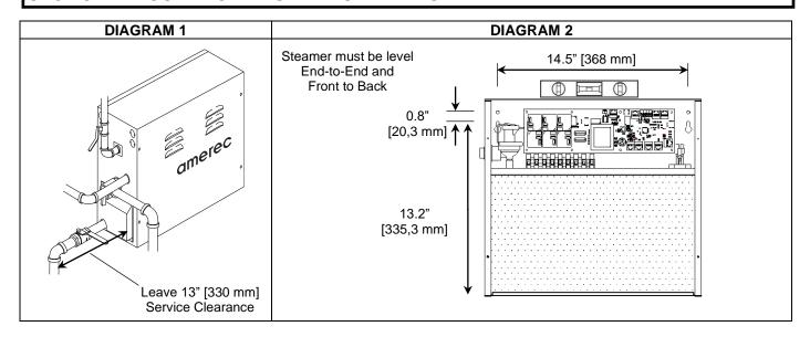
The AMEREC steam generator can be hung on a wall or sit on its base. The best mounting location will satisfy all or most of the following:
