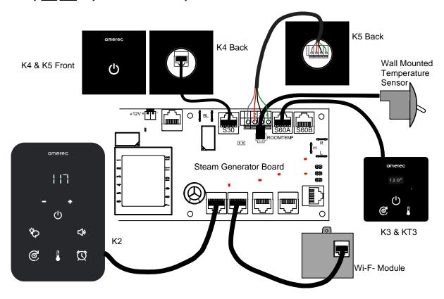
**Note**: The K2 and K3 controls provide bath temperature and run time control and they require a temperature sensor. The K4 is an on/off control used to start and stop the bath but they do not have temperature control. When using only a K4, turn the bath on when it is too cool and, if the bath becomes too hot, turn the bath off.
