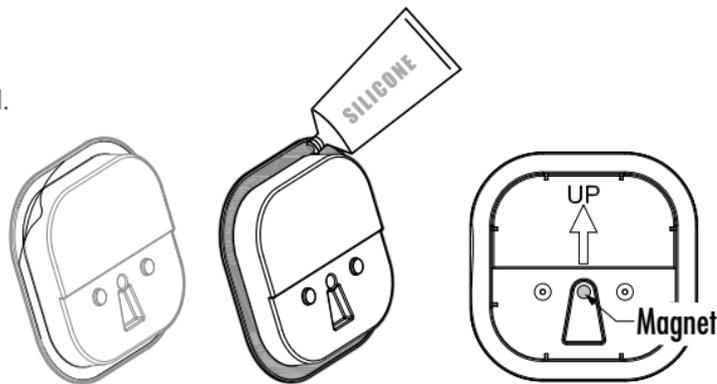
**NOTICE** Do not apply excessive amounts of silicone. Do not apply silicone to any other parts of the control including the adhesive gasket. Place the flush mount box into the hole.
