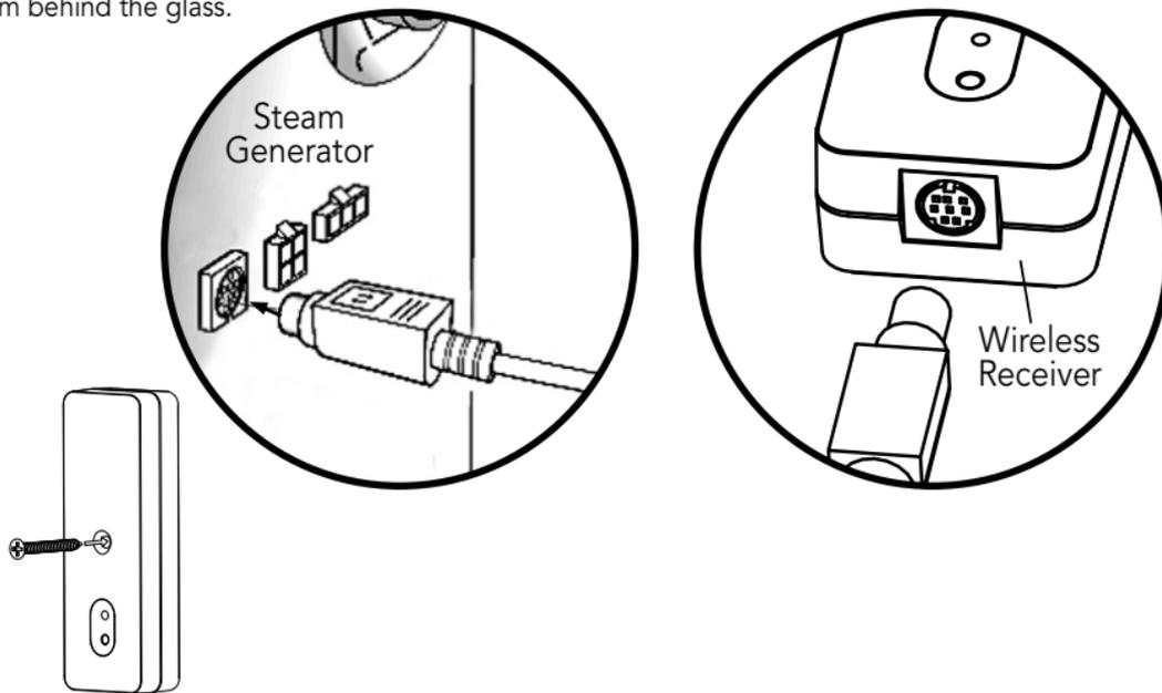
**NOTICE** Do not rest the dongle on the steam generator, the metal case of the generator may shield the RF signal.
