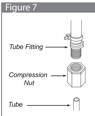
2. Clear Tubing connections: The clear tubing that is used to carry the oil to the steam line is secured with special 1/8” tubing fittings. These fittings are assembled by sliding the tube through the nut and bottoming the tube into the fitting. Then tighten the nut until the tube is secured.
