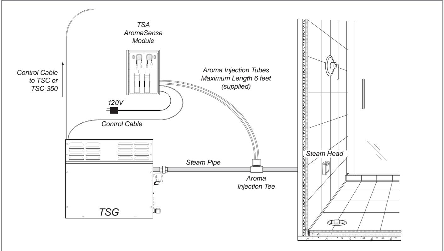
2. Make sure a 120 volt outlet is located next to the TSA AromaSense Module mounting location.
