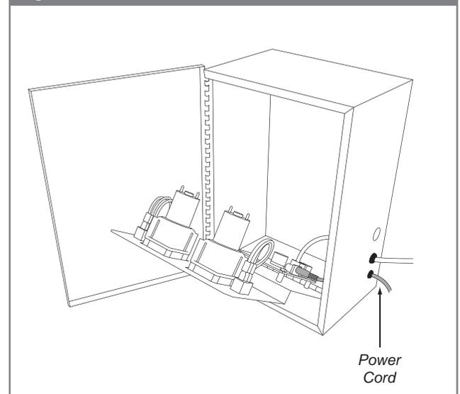
6. Plug the power cord (supplied) into the TSA AromaSense Module's circuit board (shown in Figure 4 and Figure 8) and to an outlet. Make sure the pump rollers spin (6) when the switches are pressed on the TSA AromaSense Module. If the pump does not spin check that the power supply is securely plugged into the pump control circuit board located behind the pump panel.
