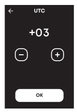
The local time zone (UTC) configuration is required if the sauna control panel has been previously connected to the Wi-Fi network.
