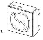
The control unit can be used to pre-set the temperature and start time of the heater and to switch the Saunum sauna climate device (hereinafter AirlQ) speed.
