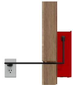
There will need to be a 1.5” diameter access hole made to run the power cable to the wall outlet.
